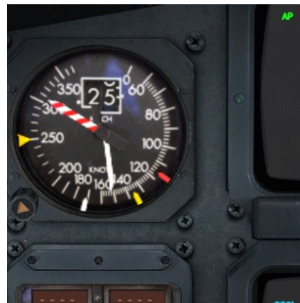
Analogue airspeed indicator
